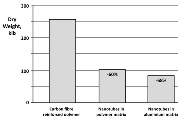
Fig. 3. Weight reduction with carbon nanotubes
