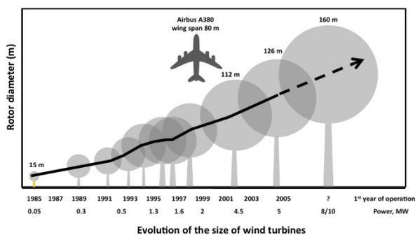
Fig. 5. Relationship between power output and wind turbine diameter
