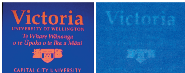
Fig. 4. Ink-jet paper printed logo with two passes of \text{Mn}^{2+} doped quantum dots (left) and with one pass of \text{Cu}^{2+} doped quantum dots (right) viewed under UV light – see ref. 3.
