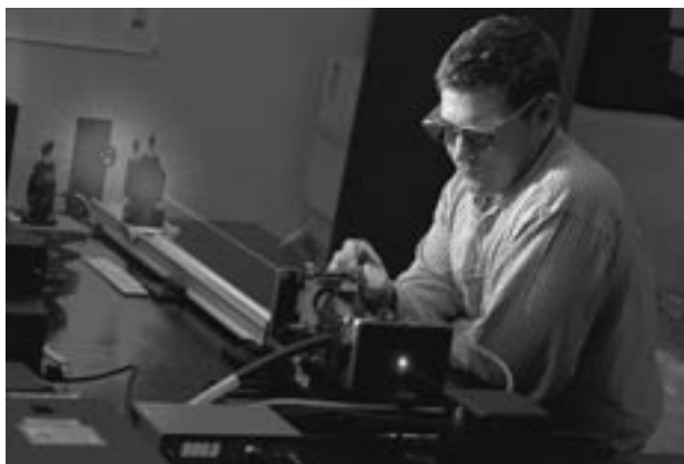
Fig. 2. The dye laser of a photoacoustic spectrometer in operation; the cavity of the laser extends from the bright spot (front) along the visible beam and the sample cell is housed in it.
