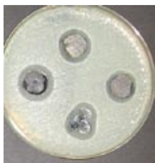
Fig. 4. Antimicrobial properties of Ag nanoparticles deposited on a cellulose fibre-conducting polymer composite; clear areas define inhibited Staphylococcus aureus growth regions.
