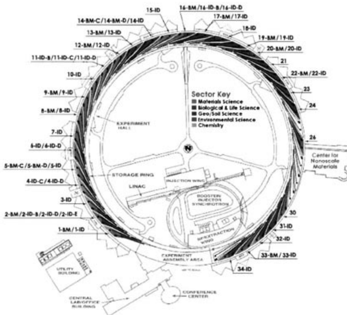
Fig. 6. Distribution of beamlines at APS Chicago; the website version of this diagram identifies the biological-life sciences (mostly protein crystallography) beamlines in blue. These now constitute around one third of the beamlines. (Taken from the APS website).
