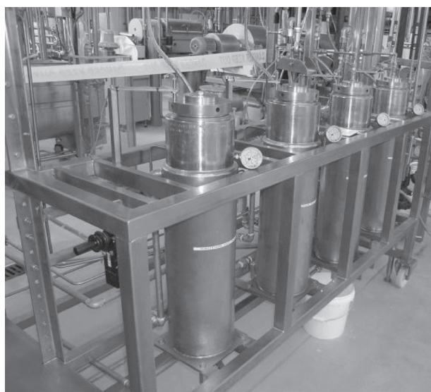
Fig. 8. Portable pilot scale supercritical fluid processing plant
