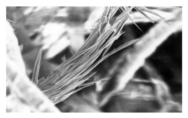
Figure 2(c) - Scanning electron micrograph of a severly mechanically disrupted fibre (ina carpet tuft), clearly showing the disintegration into cortical cells. Magnification = 800 x.
