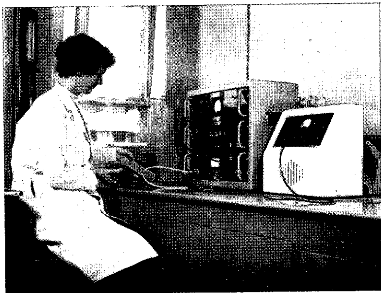
How "hot" is it? A sample is placed in the lead "castle," which contains the Geiger-Muller detecting tube, for a determination of the amount of radio-activity present.
