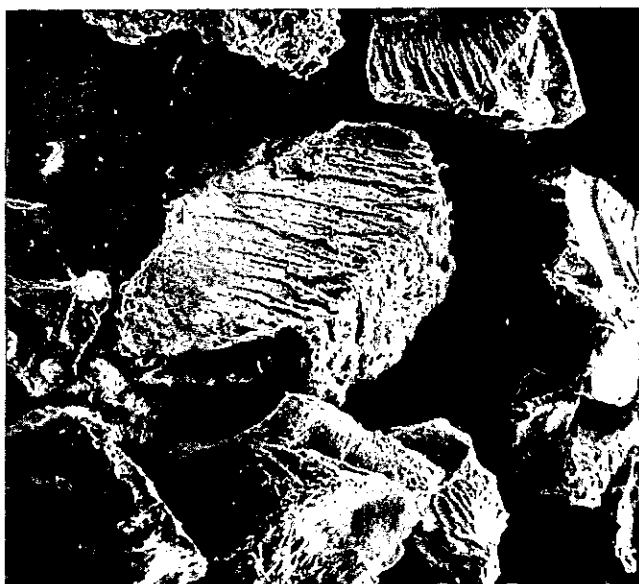
Scanning electron micrograph of a DEAE ion-exchange cellulose made, after milling, from milled viscose rayon monofilaments of large denier obtained from the Asahi Company in Japan. The rough and smoother fracture surfaces are similar to those across and along the grain in wood samples. The preferred alignment in the viscose may be due to the manufacturing extrusion process. Magnification 175x.
