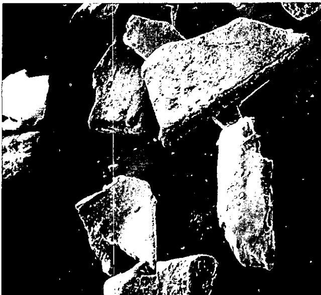
Scanning electron micrograph of a DEAE ion-exchange cellulose made, after milling, from viscose obtained from the Viscose Development Corporation. The laminar structure of the flake viscose is preserved in exchanger. Magnification 33x.
