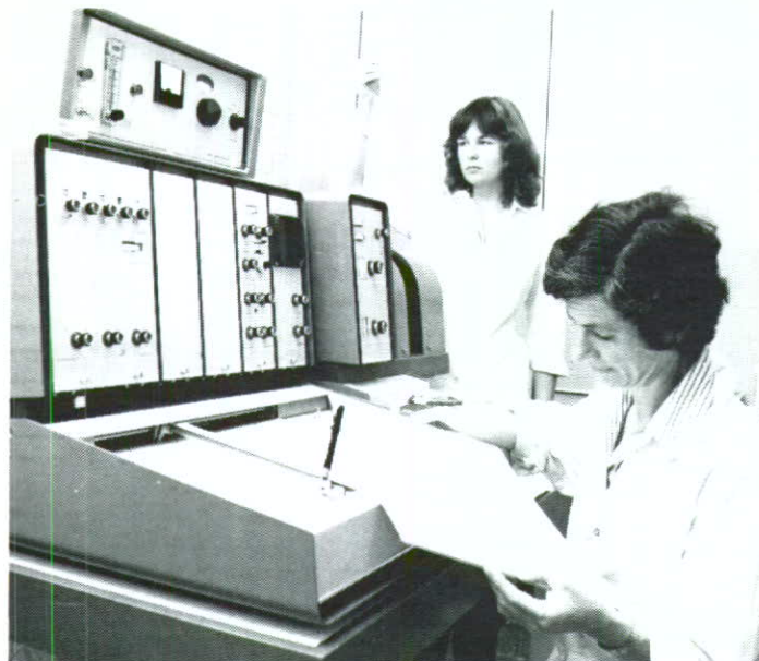
Figure 1. A Varian E-104A ESR spectrometer. Miss V. Ritchie is about to insert a sample into the sample cavity. Mrs J. Husbands examines a spectra.
