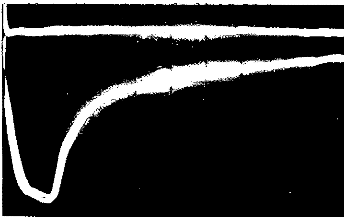
Fig. 5. Time course of the absorbance change at 400 nm during the actinidin-catalysed hydrolysis of Z-Lys ONp at pH 7.0. Vertical scale: 0.01 absorbance units per div., horizontal scale 5 ms per div. Three reactions are superimposed.
