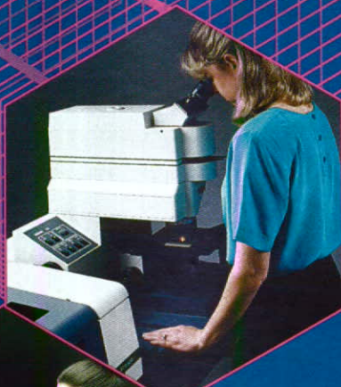
Bio-Rad commercialized the FT-IR microscope, and now offers the UMA 500 research system with fingertip controls.
