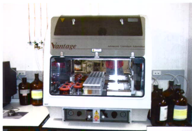
Figure 9. The Advanced Chemtech 390 automated peptide and small molecule synthesizer.
