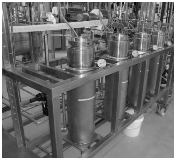
Fig. 8. Portable pilot scale supercritical fluid processing plant
