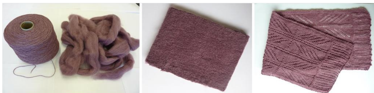
Fig. 4. Purple nanogold–wool composites produced with AuNPs. Reproduced with permission from ref. 16. © 2011 Johnston and Lucas.
