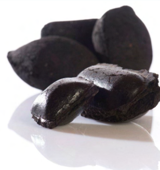
Torrefied, densified Pinus radiata wood briquettes prepared at Scion
